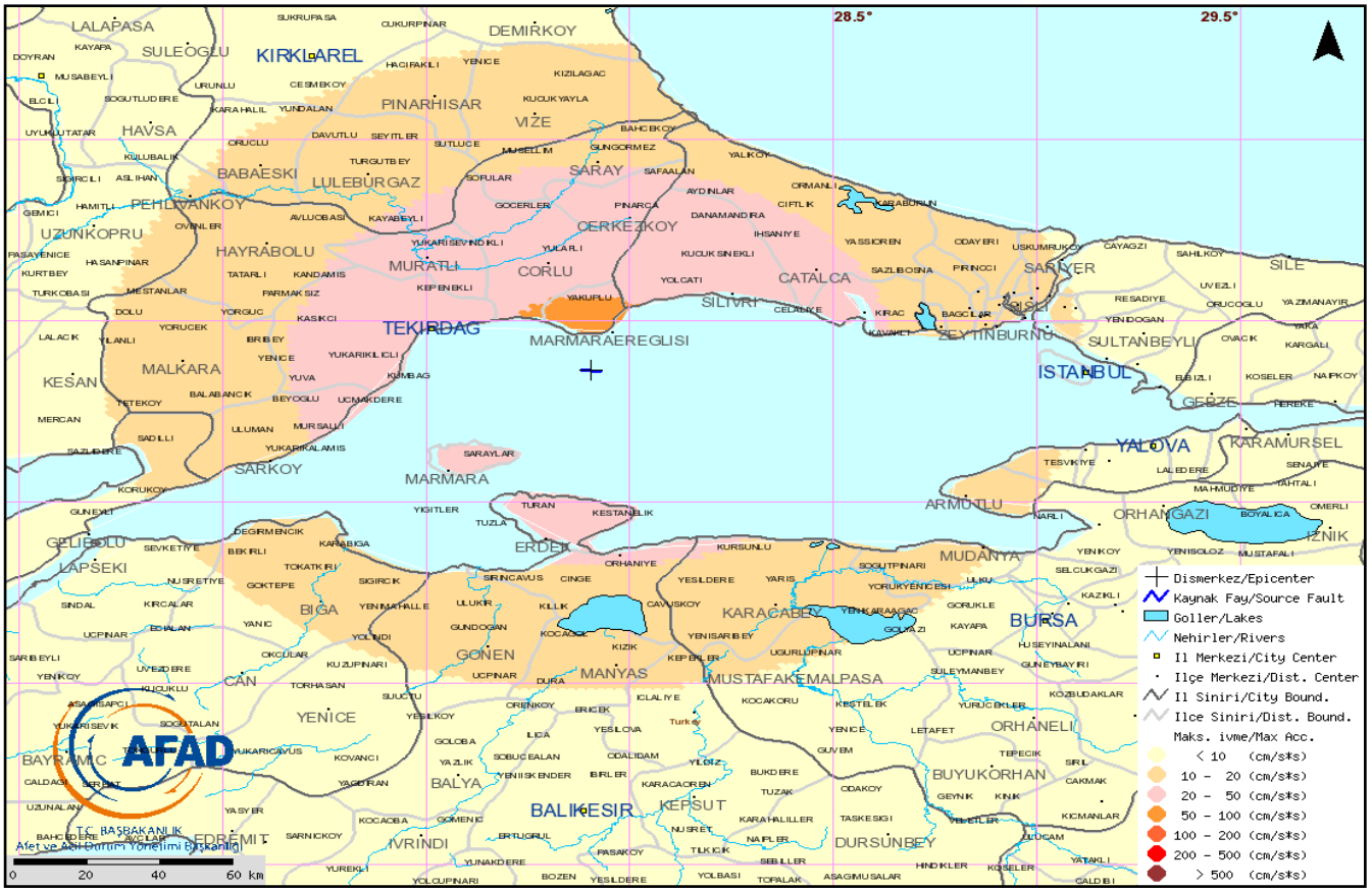
Fig.7. Peak Ground Acceleration Distribution of Marmara Sea Earthquake (MI=5.1)
